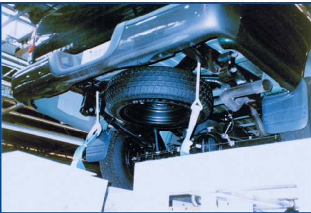
L.S.P.V adjustment system Applies specified load on the assembled vehicle and adjusts the L.S.P.V (Load Sensing Proportioning Valve).
