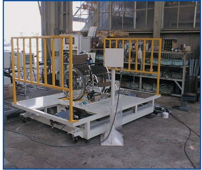
Simulates road driving conditions for motor drive wheelchair to perform various kinds of tests.
