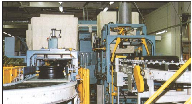
TIRE AND WHEEL CONVEYOR
